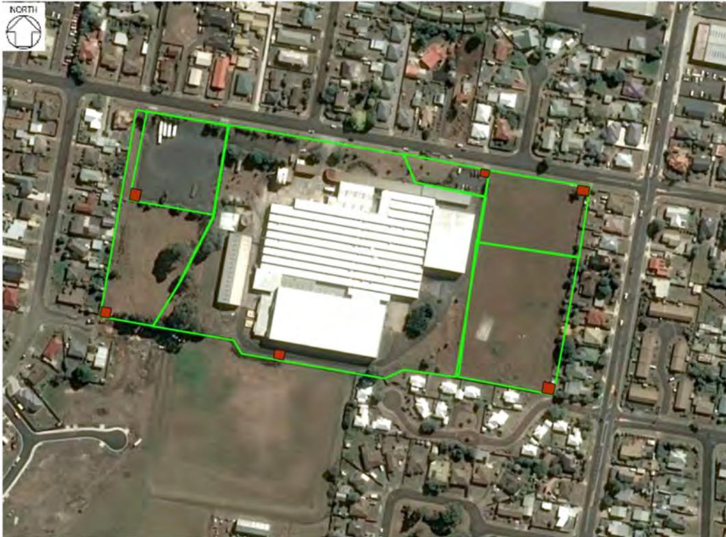
Figure 4: Assumed Existing Catchments with Assumed Points of Discharge
