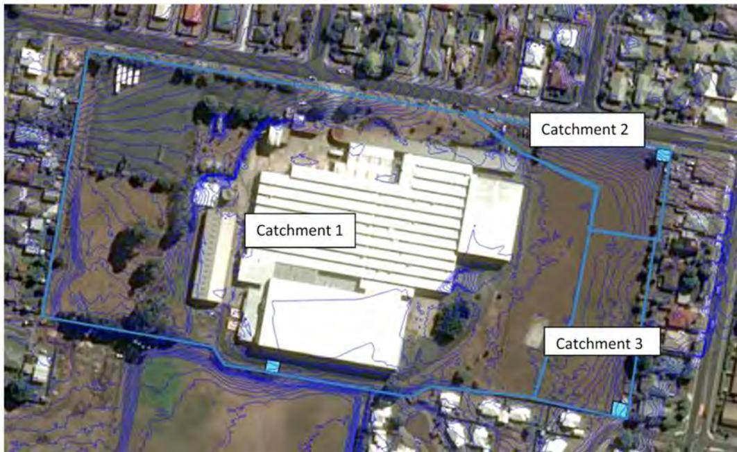
Figure 7: Scenario 2 Design Catchments and Discharge Locations
