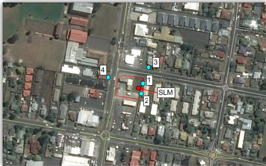
Figure 1 – Aerial view of the 110-118 William St petrol station redevelopment site and surrounding area with the monitoring and receiver positions marked.
