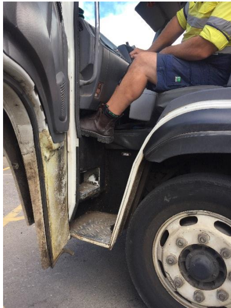
Photo 1: Photo of the 'low entry door' on the existing garbage truck
