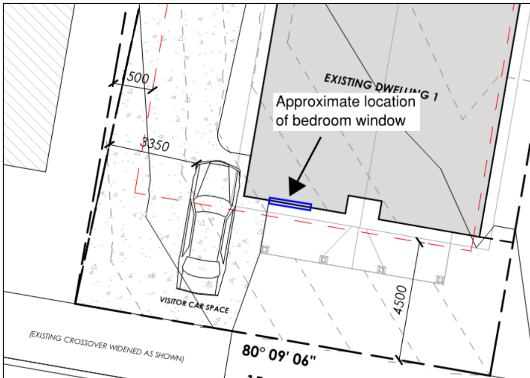
Figure 7 – Location of bedroom window adjacent to visitor carparking space (n + b, 2018)
