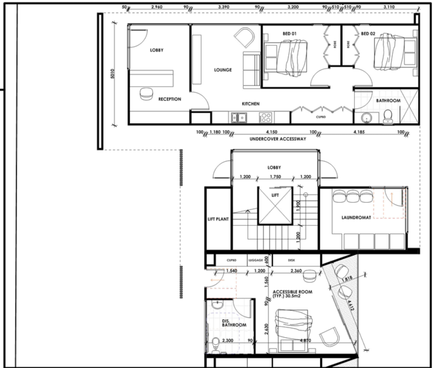
GROUND FLOOR PART PLAN SCALE 1:100 Project North 0mm 1000 2000 3000 4000 5000
