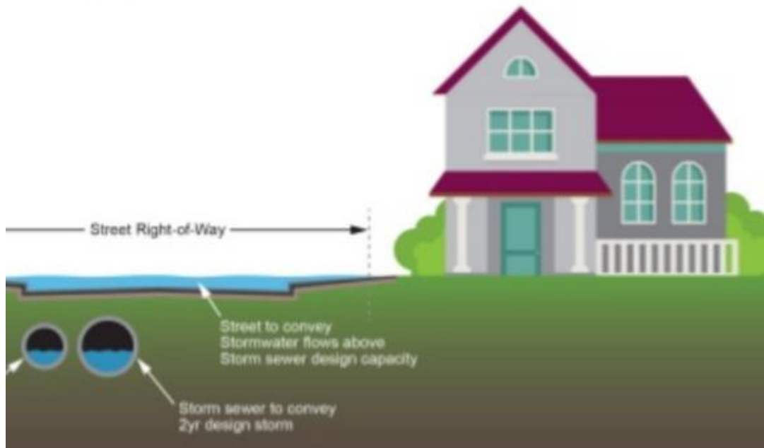
Figure 2: major and minor stormwater systems
