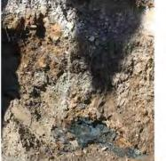
A black oil soaked patch of clay on the south face of the pit can be seen on the bottom of the photo. Sample UST-B1-1.7m was taken from this area.
