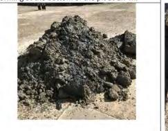
The oil soaked clay was heaped into a separate stockpile for disposal. Samples ST1-3 were taken from this stockpile. Note the oily black appearance of the clay.
