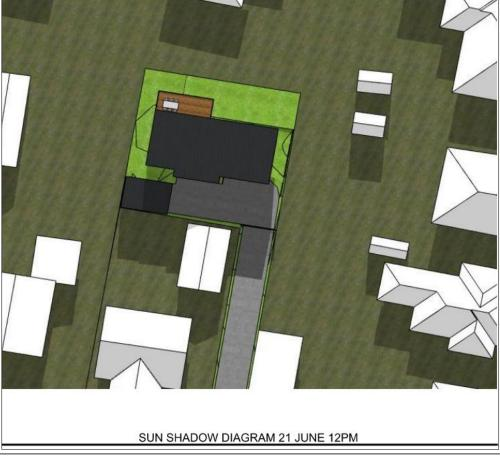
Figure 18 – Shadow diagrams June 21 12PM (Cykel Architecture, 2023)
