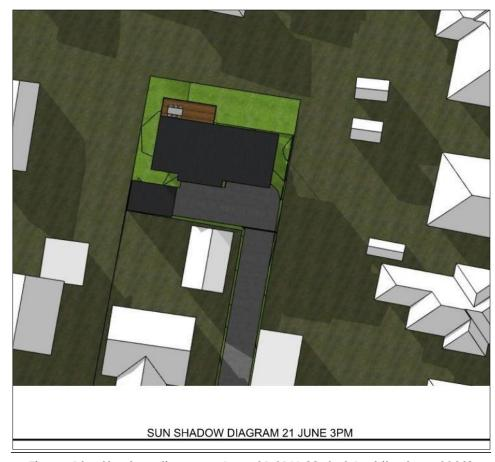
Figure 19 – Shadow diagrams June 21 3PM (Cykel Architecture, 2023)
