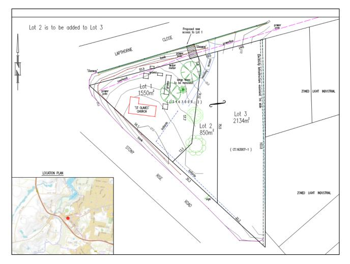
Figure 9 – Boundary adjustment plan (Michell Hodgetts Surveyors, 2022)
