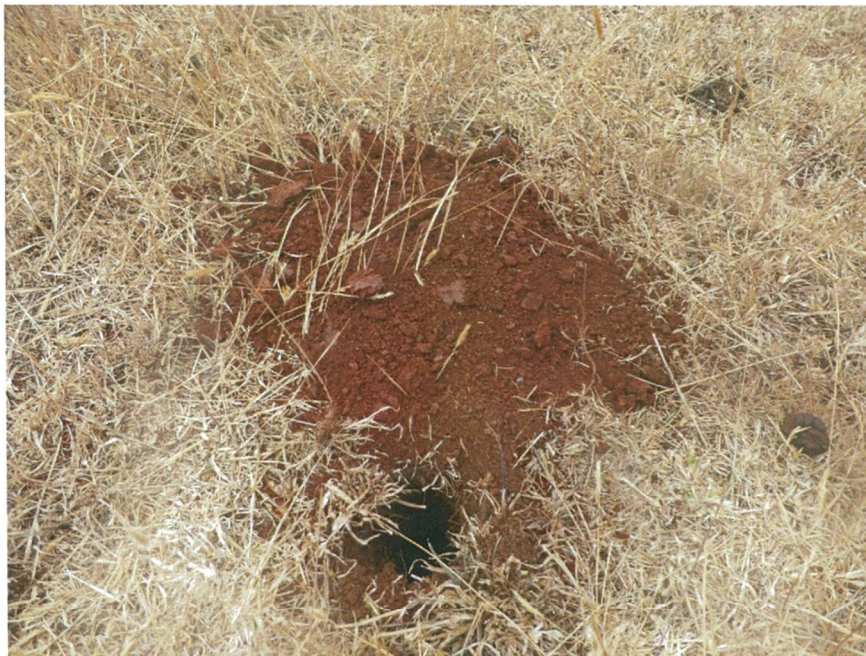
Photograph W4 – Excavated material from test hole. Note friable consistency with little moisture
