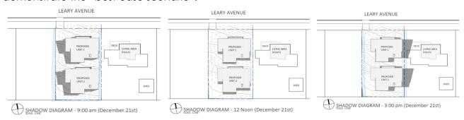
Figure 9 – Shadow diagrams for unit development on 21 December (Source: Supplied – PA2019.0149).
